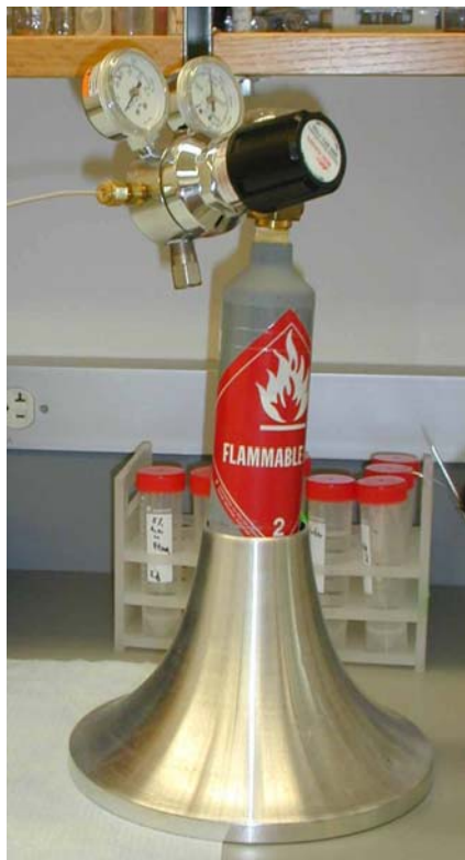
Holder Available from Sima appropriate for in-use or in storage lecture bottles
