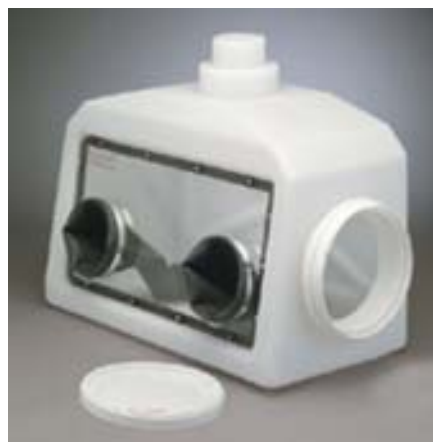
Glove box with venting capability
